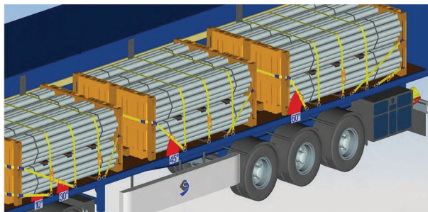
Protecting the cargo during movement (combination): forward, sideways and backward – with the use of a pallet with a non-slip surface.
